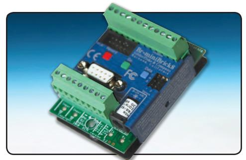
The **Br-miniBrick8** is a complete stand-alone Show Control System. It features two 'trigger' inputs, DMX-512 input or output, two airplane-style servo motor control outputs and eight high current outputs for driving solenoids, lights and relays.
